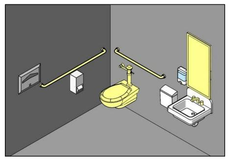
In a restroom project involving alterations to the toilet, grab bars, faucet controls, and mirror, the standards apply to these elements but not to those that remain unaltered. In more extensive projects where additional elements are altered, application of the standards is greater, commensurate with the scope of work.
