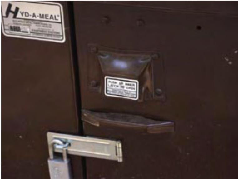
The latch hardware is sturdy and appears to be panic-operable from inside. The latching mechanism is all exposed to view inside the door, which will likely facilitate maintenance over time. The doors have a cable which keeps them from being over-opened, a feature not seen on other models.
