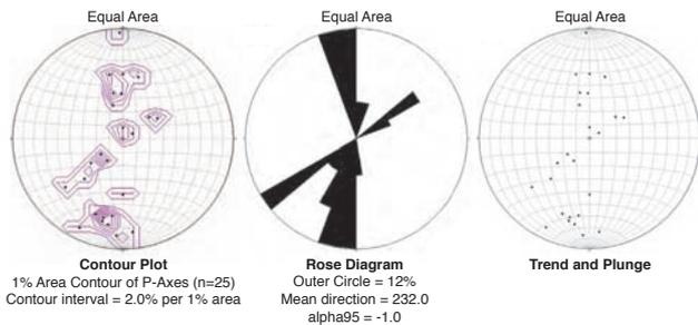
**Fig. 8.** Contour plots, rose diagrams, and trend and plunge data for joint surfaces at Staircase Falls rock fall detachment area ( $n=25$ ) (see Table 1 for data). More joints exist than were measured.
