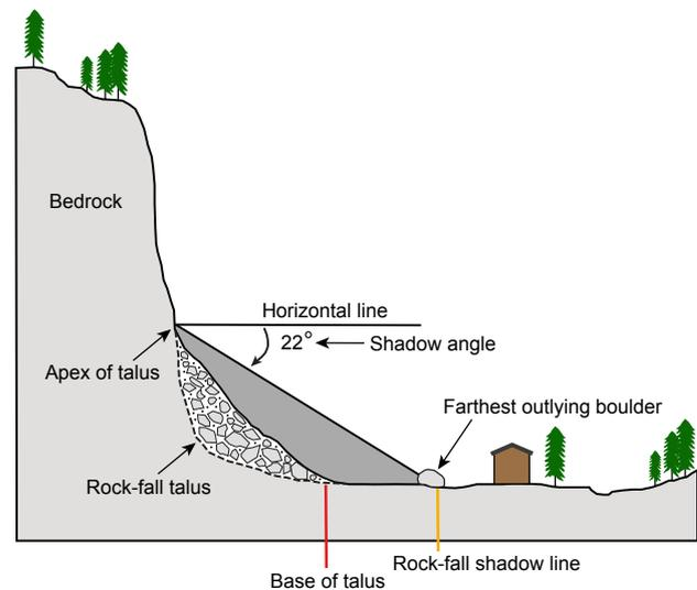
**Fig. 9.** Schematic of rock-fall talus slope, base of talus (red line), and farthest outlying boulder, illustrating determination of rock fall shadow angle and shadow line (orange line); after Wiczorek et al. (1998, 1999), modified from Evans and Hungr (1993).
