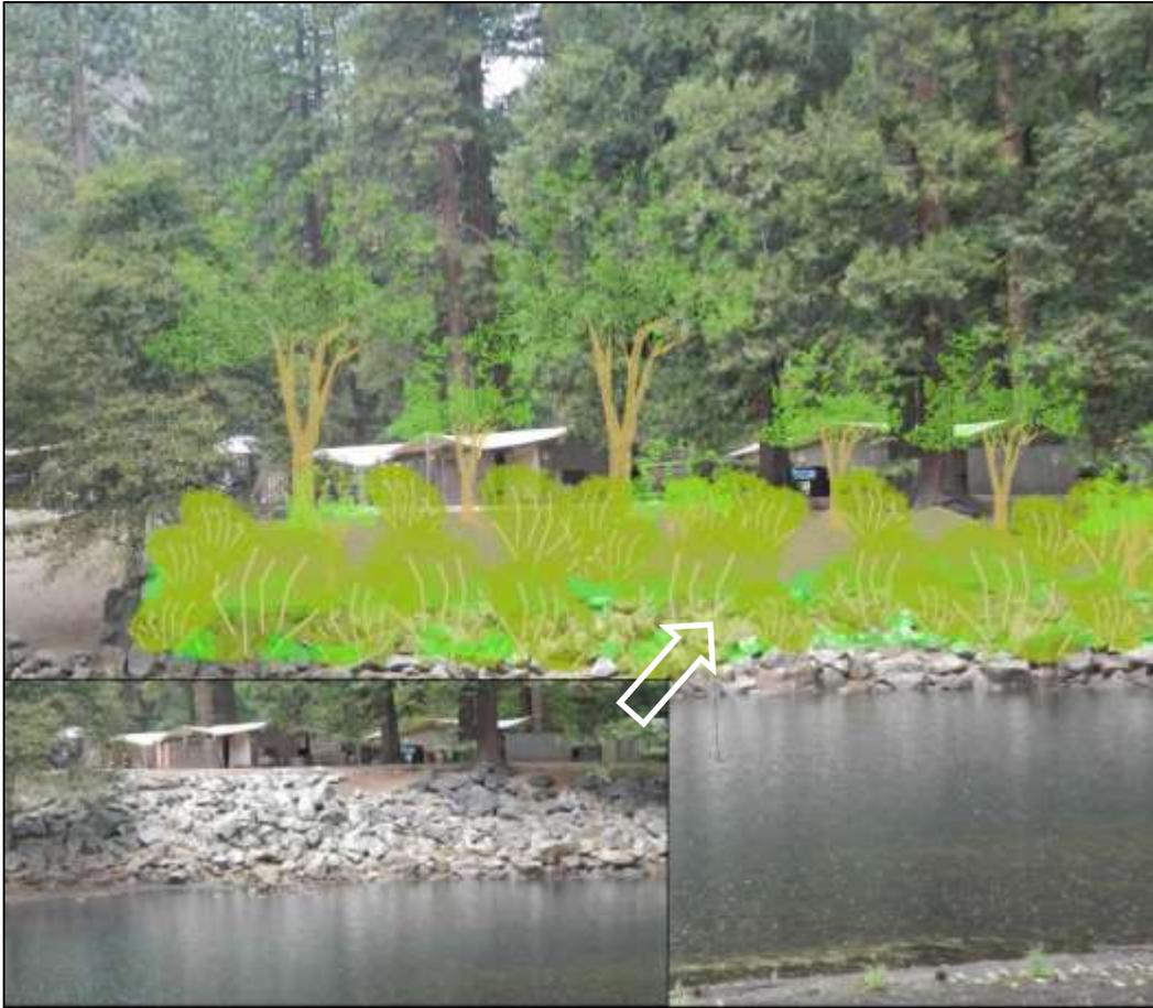
**Figure 6.** Diagrammatic view of vegetative bank reinforcement, with or without initial removal of existing riprap.
