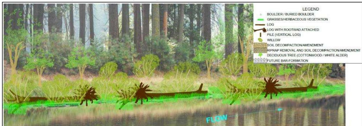
**Figure 8.** Reinforcement and rebuilding of trampled banks, plus riparian vegetation replanting within and above the bank structures.
