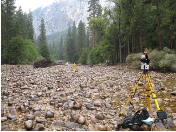
(A) D50 grain size: 83 mm
