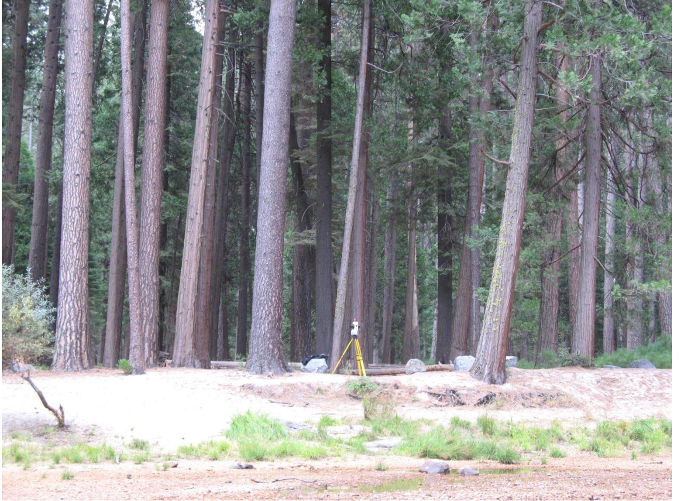
Figure 2. Photograph of ground-based LiDAR unit on river left streambank approximately 100 m downstream of Ahwahnee Bridge at site of the previous Lower Pines Campground. Note the extensive and large coniferous forest with relatively sparse riparian growth and exposed streambank sediments. Photograph taken by J.T. Minear, 9/21/2007.
