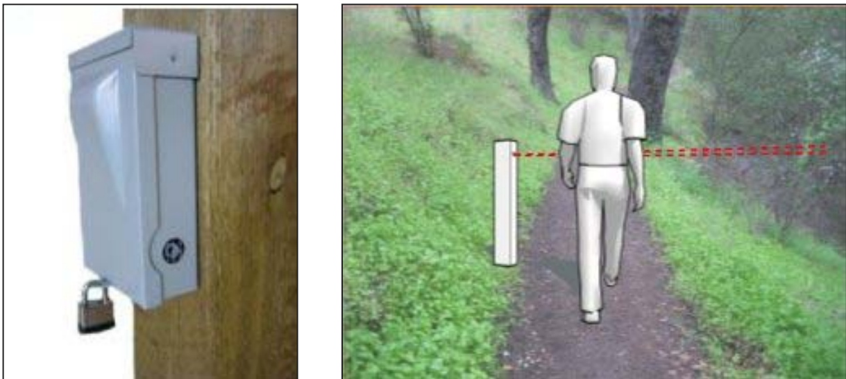
Figure 2. TRAFx visitor counter in lock-box (left) and conceptual example of counter in operation (right).
