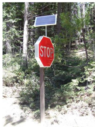
**Figure 3-38 – Solar-powered Sign at South Entrance**
