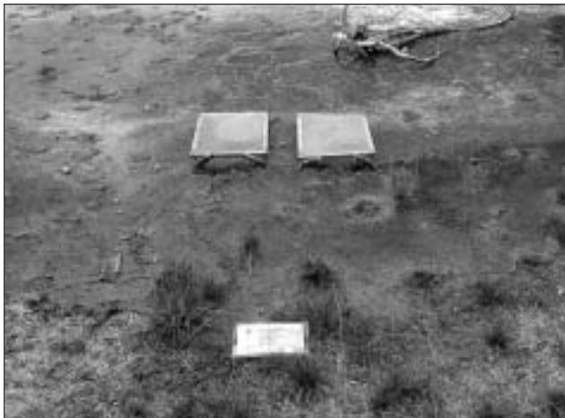
Screens used to shade a microbial mat from ultraviolet rays at Octopus Spring. One of many research projects undertaken by researchers from outside the NPS.
