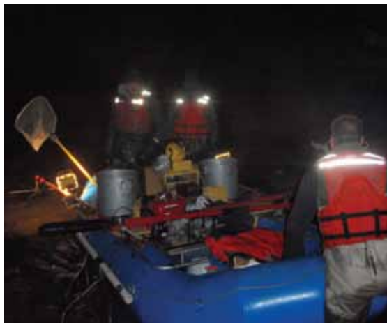
Raft outfitted with electrofishing equipment.
