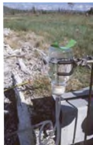
Figure 4. Field-portable, bubble-stripping apparatus for measurement of H_2 in geothermal waters. An intake tube is wrapped in insulation to keep the water hot. A peristaltic pump pumps water through a glass jar (right) with a 20-ml atmospheric air bubble inside. After an amount of pump time at a given rate of flow, the bubble is withdrawn for analysis.
