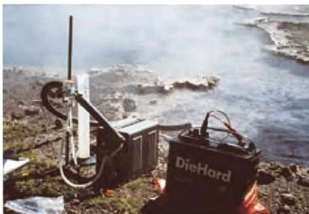
Figure 4. Field-portable, bubble-stripping apparatus for measurement of H_2 in geothermal waters. An intake tube is wrapped in insulation to keep the water hot. A peristaltic pump pumps water through a glass jar (right) with a 20-ml atmospheric air bubble inside. After an amount of pump time at a given rate of flow, the bubble is withdrawn for analysis.
