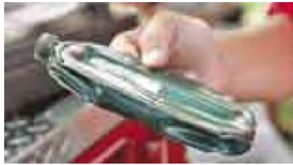
An empty, crushed steel canister.
