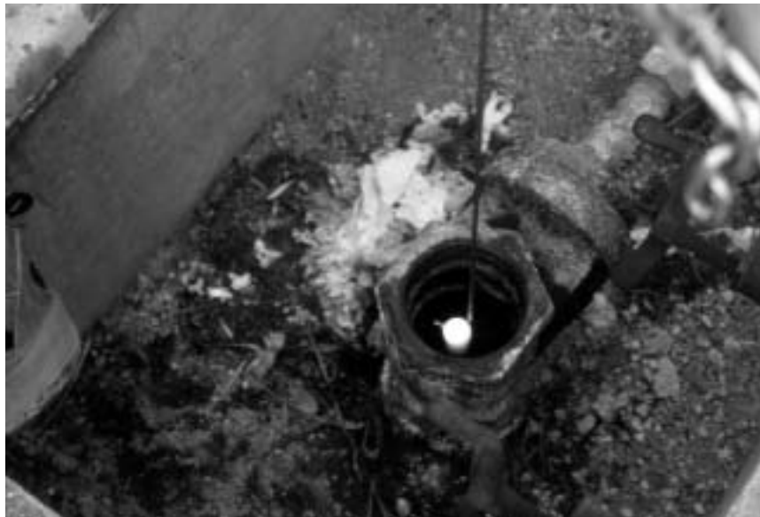
Figure 4. Cable with attached vials is lowered into the well.
