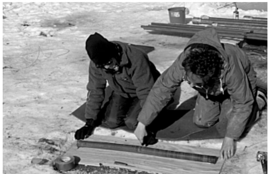
Cathy (on the left) examines a section of core removed from the bottom of Crevice Lake. This piece of core will be carefully packaged in plastic wrap and aluminum foil and then sent on to a laboratory for further analysis. NPS photo.
