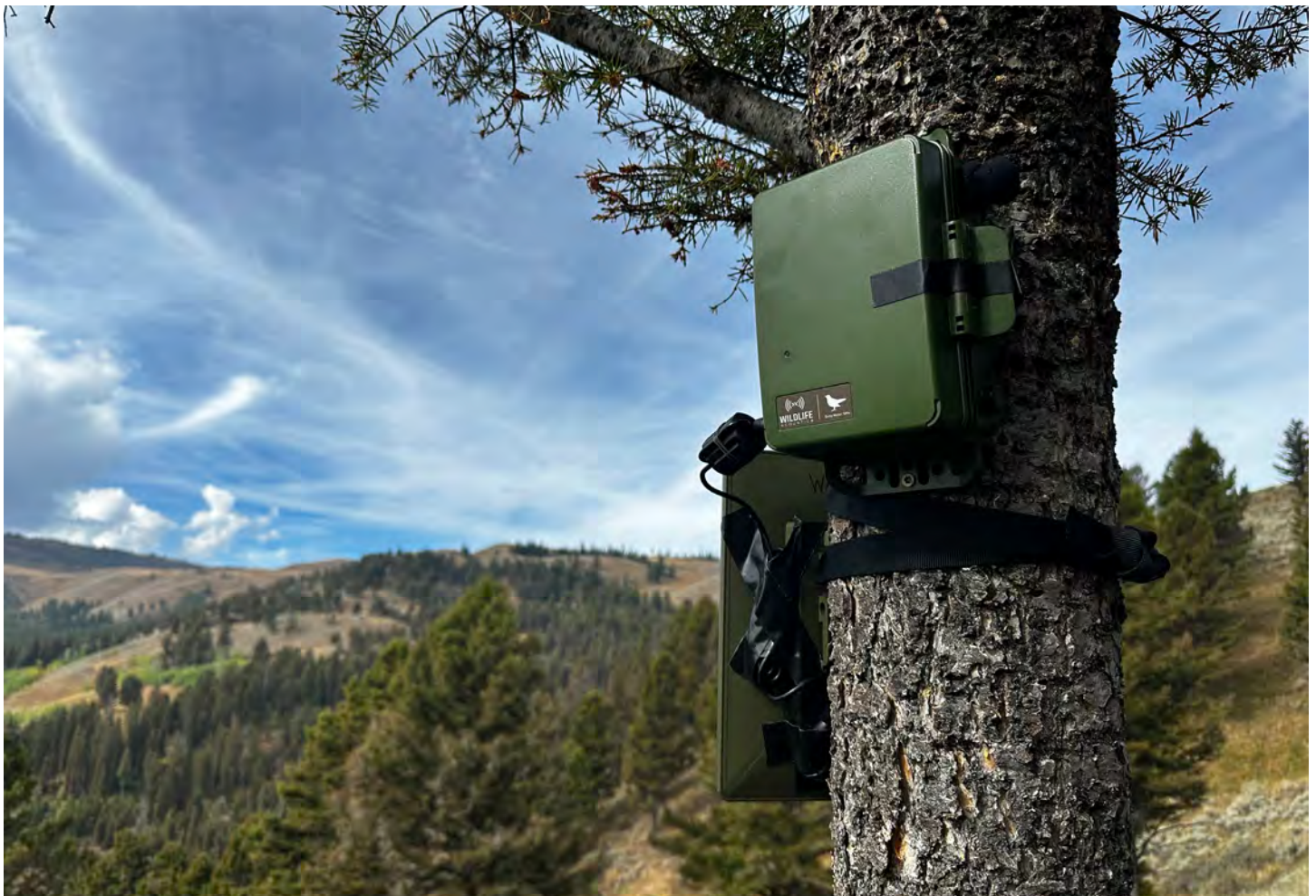
Solar-powered ARUs like this one are part of an expanding effort by the Wolf Project to implement non-invasive monitoring tools to study wolves. Data from these units will feed into wolf population and behavioral monitoring studies, as well as provide general Yellowstone soundscape data that can be used in a variety of other studies. (D. Stahler/NPS photo)
