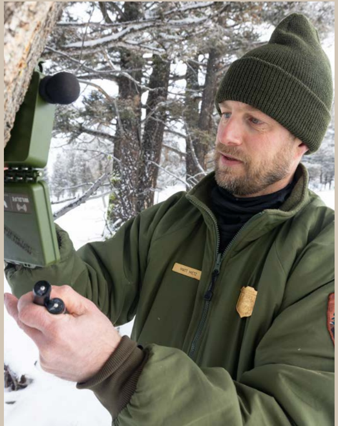
Project Biologist Matt Metz services an autonomous recording unit as part of the wolf bioacoustics study. These devices record Yellowstone's soundscapes 24/7 with the goal of detecting wolf vocalizations to use as a passive monitoring tool and to study wolf communication. NPS PHOTO: J. Frank
