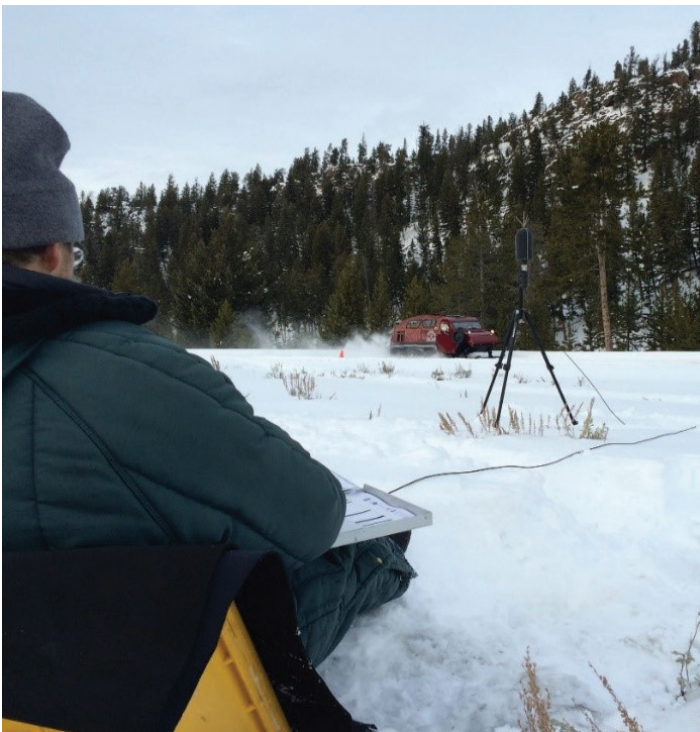
Researcher conducting snowcoach sound testing. - NPS Photo
