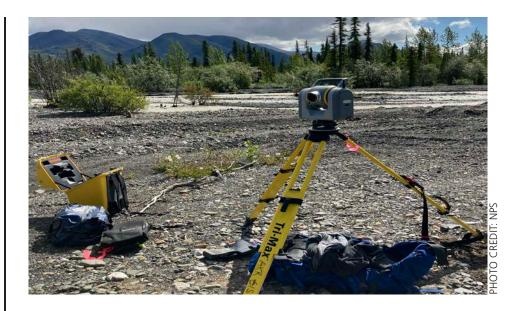
Pictured above is the SX10 terrestrial LiDAR Scanner used on Lost Creek in 2020.
