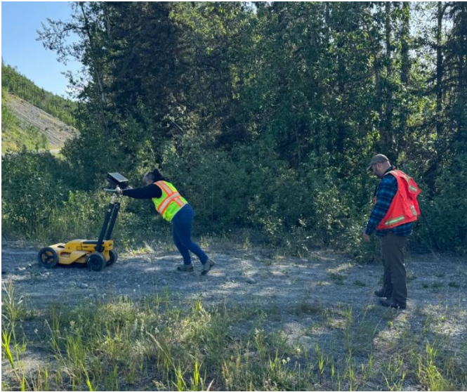
NLURA Staff conducting GPR surveying at Squirrel Creek
