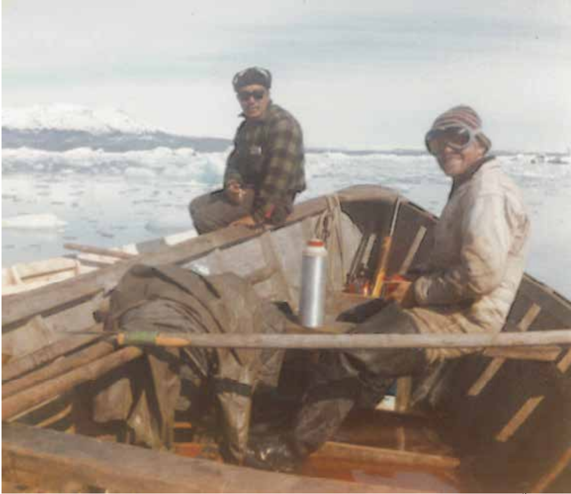
Figure 10 – An example of a Yakutat seal hunting boat, as they appeared in the mid-20 th century. Made of planks, these boats were heavily reinforced with extra planks, tires, and other items to reduce damage to the hull from floating ice. Photo courtesy of Skip Johnson.
