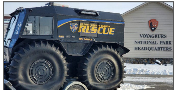
A sherp ATV used by the St. Louis County Sheriff's dept for search and rescue operations was on site during training.
