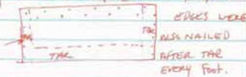
Pitch of the roof 5-6/12 made for difficult application and unevenness of sheathing below caused roll roofing to not lay flat along entire section. As a result tar oozed out in areas, but it would rather have over tarred roofing than under tarred it.
