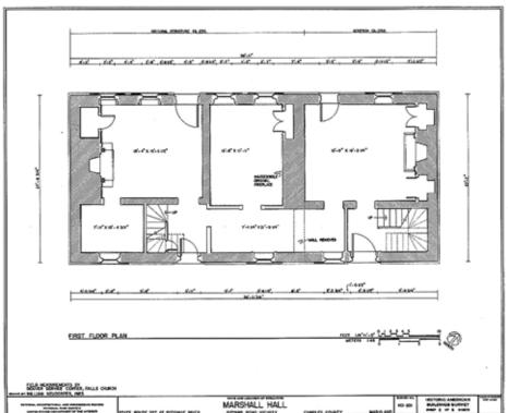
Figure 10. Marshall Hall, Charles County. Northwest elevation drawing and first floor plan, drawn by Paul D. Dolinsky and William Neudorfer, respectively, 1983. Around 1760, the Marshall family enlarged a circa-1725 five-bay, one-and-a-half-story brick house by adding an attached kitchen with living quarters upstairs (at left in top drawing).
