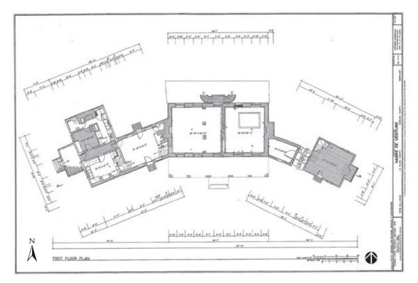
Figure 22. First floor plan of Haberdeventure, 1985. The east wing is on the right; the west wing is on the left.
