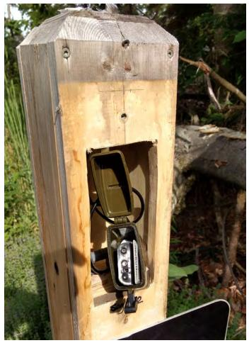
Figure 10-1: An example of a trail counter hidden within a sign post at Sleeping Bear Dunes National Lakeshore in Michigan; sign was turned upside down to expose the counter for the photograph. (Source: NPS)
