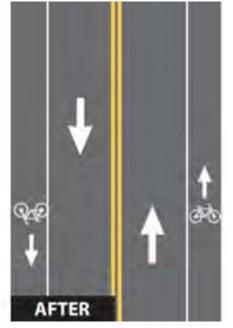
Figure 4-11: Before and After Road Diets. (Source: FHWA)
