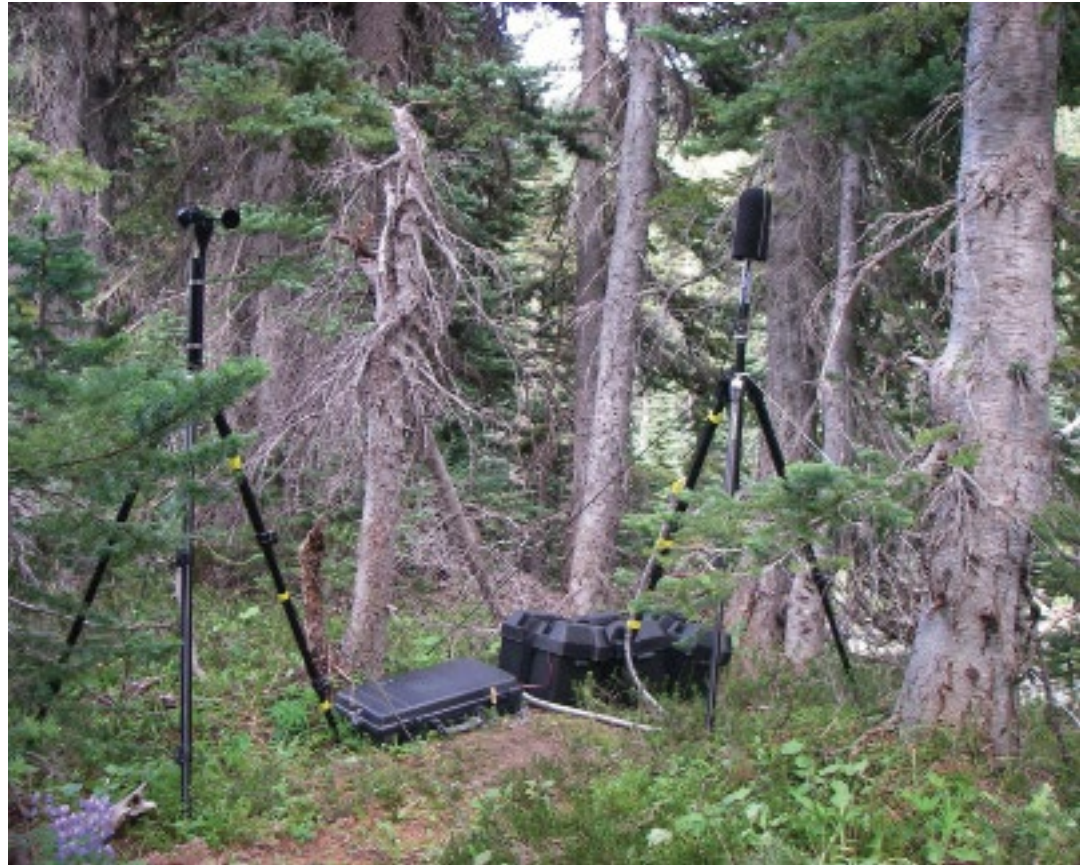
Sound monitoring equipment at Mount Rainier National Park collects data for approximately 25 days. NPS photo.
