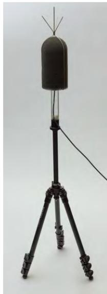
Figure 4.2: Assembled microphone tripod
