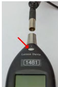
Figure 4.7: Microphone cable connection to the LD831
