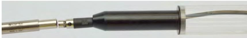
(c) Aligning the preamplifier
