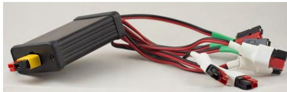
Figure 4.4: Battery bank connector, a.k.a. “battery squid.”
