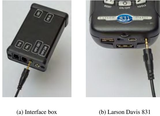
Figure 4.6: Audio connection between interface box and LD831
