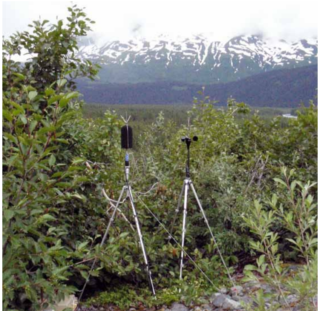
Acoustical monitoring station in Kenai Fjords National Park
