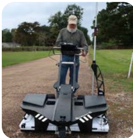
Dan Elliot operating the “Stream C” compact array ground penetrating radar system.
