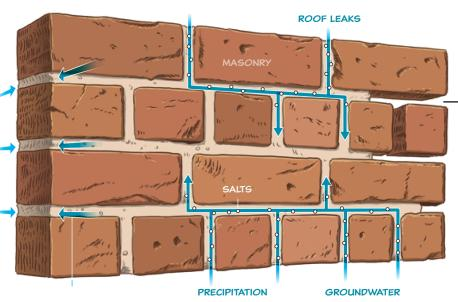
SINCE MORTAR IS REPLACEABLE, A PROCESS CALLED REPOINTING, IT SACRIFICES ITSELF FOR THE GOOD OF THE SYSTEM. BUT FOR THE SYSTEM TO WORK, THE MORTAR HAS TO BE SOFTER THAN THE MASONRY IT HOLDS TOGETHER
