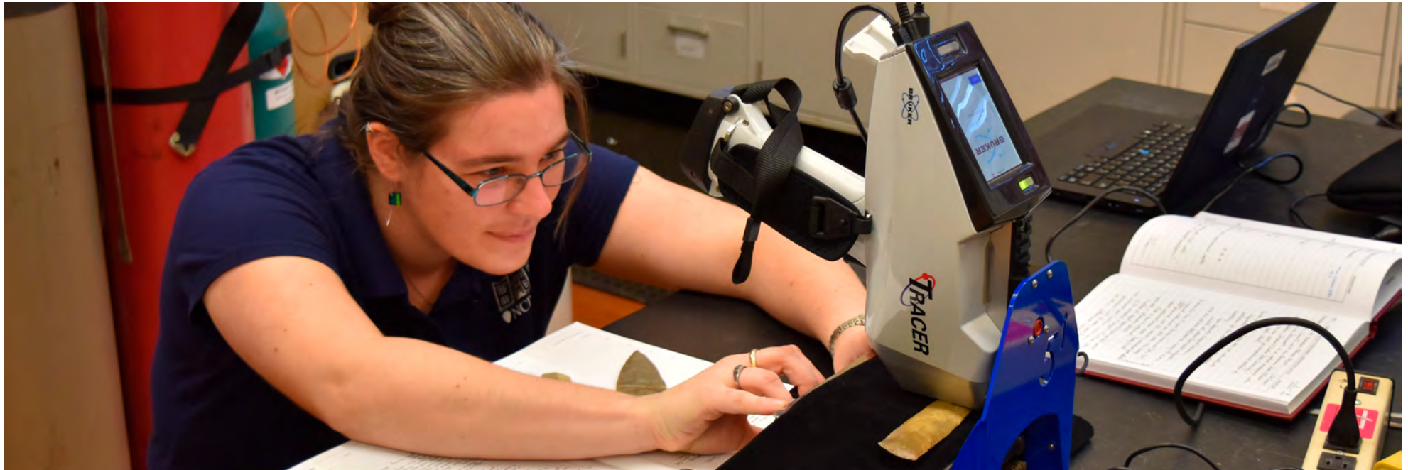
Catherine Cooper, Research Scientist, studies archaeological objects using a portable X-ray fluorescence analyzer.
