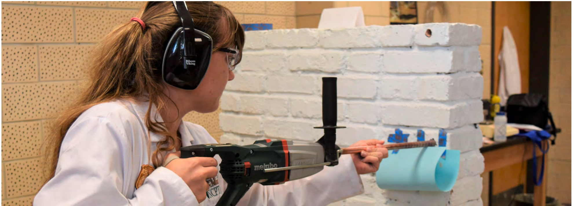
Marrissa Bartz, Research Associate, drills samples for testing salt content within the test walls.
