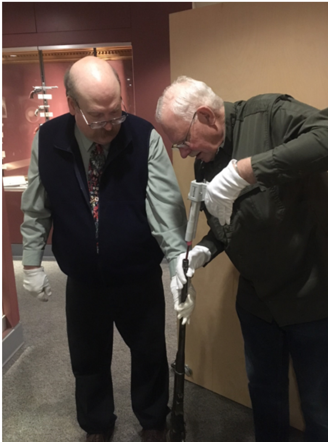
Dr Doug Scott with assistant taking an epoxy impression of the rifle barrel
