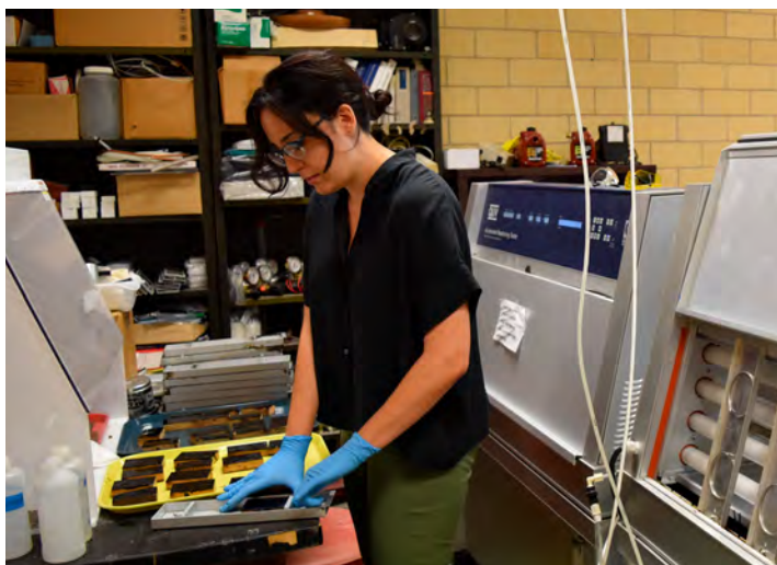
Elizabeth Salmon, Research Associate, prepares oiled brick samples for artificial weathering
