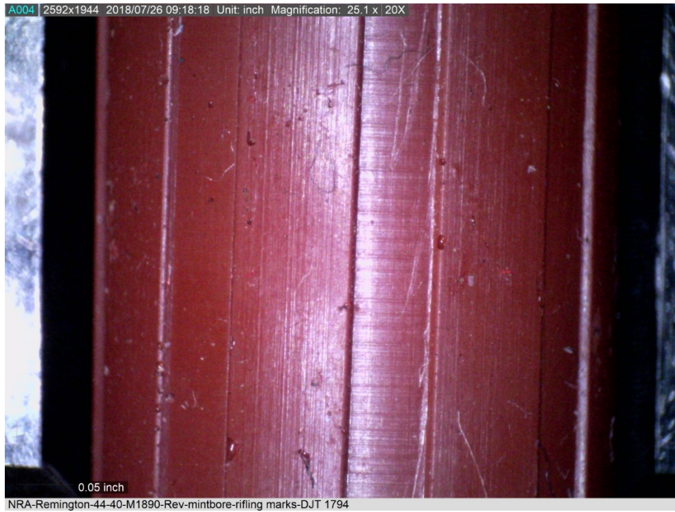
Figure 16. Digital microscope image of a Model 1890 Remington .44-caliber revolver barrel cast illustrating a near perfect bore. Note the rifling is right hand twist and the lands and grooves are flat.
