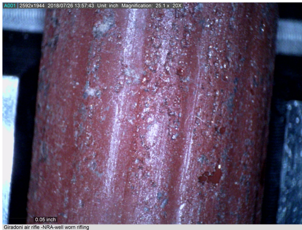
Figure 17. Microscope image of well-worn rifling with rounded grooves in a Giradoni air rifle similar to the type carried by William Clark on the Lewis and Clark Expedition. Note the rusty condition of the rifling reflected in the cast which makes precise measurements more difficult but not impossible to obtain.
