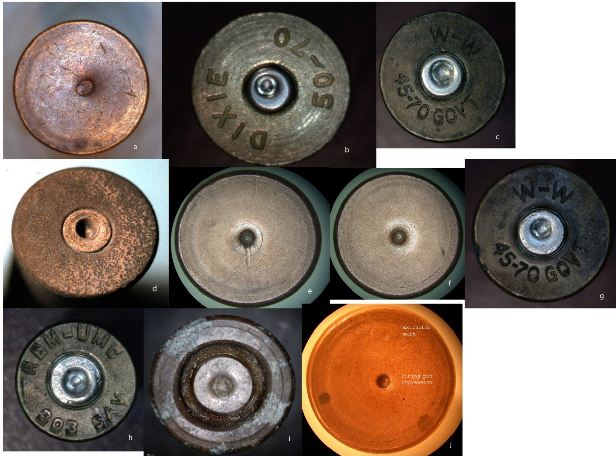
Figure 20. Centerfire firing pin impressions which are commonly hemispherical and similar in configuration. The means to determine firearm type includes analysis of the firing pin shape and the location and type of extractor and ejector marks. a. Colt Model 1873 .45-caliber revolver, b. Gatling gun, .50-70-caliber revolving barrel artillery gun, c. Phoenix, .50-70-caliber rifle, d. Remington .50-70-caliber rolling block rifle, e. Sharps, .50-70-caliber rifle (note the firing pin drag mark which is typical of the Sharps drop action), f. Springfield Model 1873, 1877, 1879, and 1884 45-70-caliber “trapdoor” rifle, g. Starr .44-caliber centerfire conversion carbine, h. Smith and Wesson No. 3, .32-caliber revolver, i. Smith and Wesson .45-caliber Schofield revolver, j. Ward Burton .45-70-caliber bolt action rifle.
