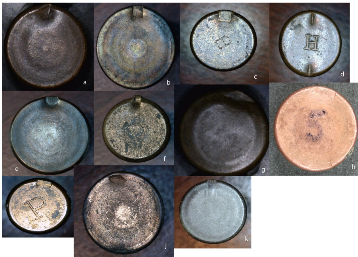
Figure 21. Rimfire firing pin impressions. a. Ball carbine .52-caliber, b. Ballard carbine .54-caliber, c. Colt Model 1872 Open top .44-caliber revolver, d. Henry and Model 1866 Winchester .44-caliber rifle, e. Jocelyn .52-caliber carbine, f. Remington .44-caliber revolver, g. Spencer 56-56 and 56-50-caliber rifles and carbines, h. Starr .54-caliber carbine, i. Smith and Wesson .32-caliber revolver, j. Warner .50-70-caliber carbine, k. F. Wesson .44-caliber rifle.
