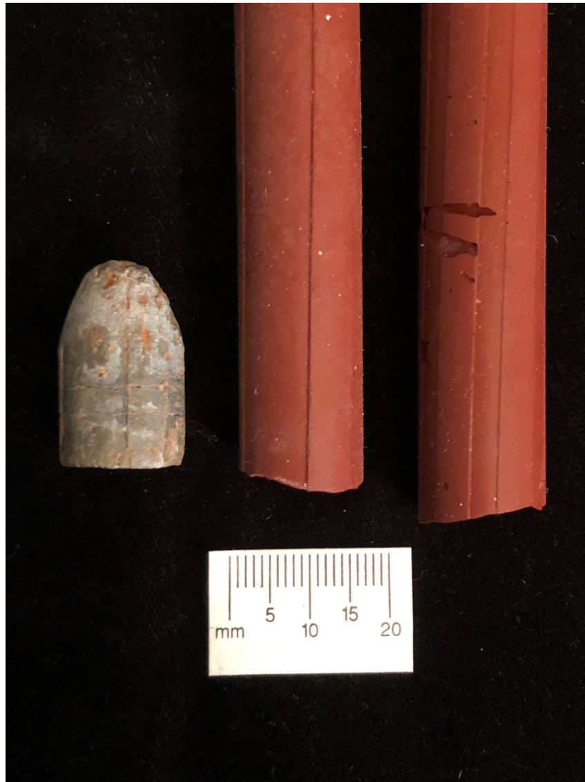
Figure 18. A .58-caliber Minié ball fired from a Pattern 1853 Enfield compared to an original Pattern 1853 and a reproduction Pattern 1853 bore casts. The bullet has a 3 right land and groove configuration. The middle cast is also a 3 right land and groove configuration while the right cast from the reproduction rifled musket is a 6 right land and groove configuration. The bullet is consistent with the original Pattern 1853 Enfield rifled musket.
