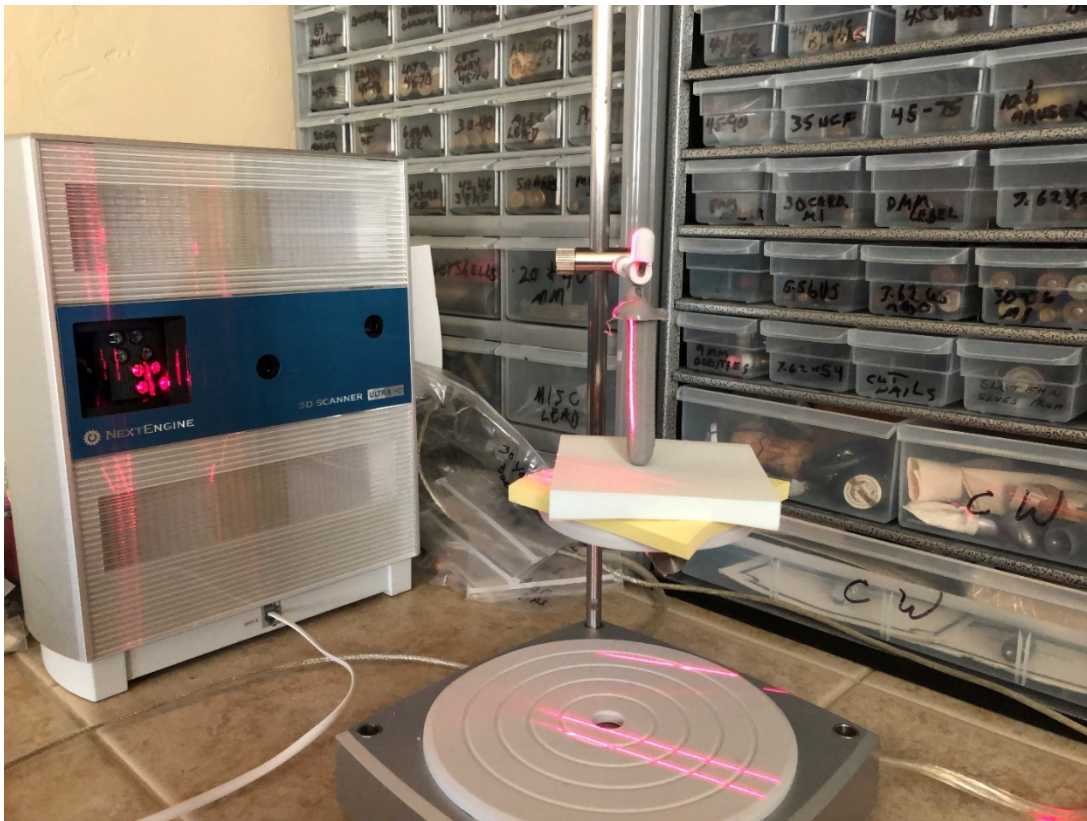
Figure 13. NextEngine scanner during the process of scanning a rifling cast.
