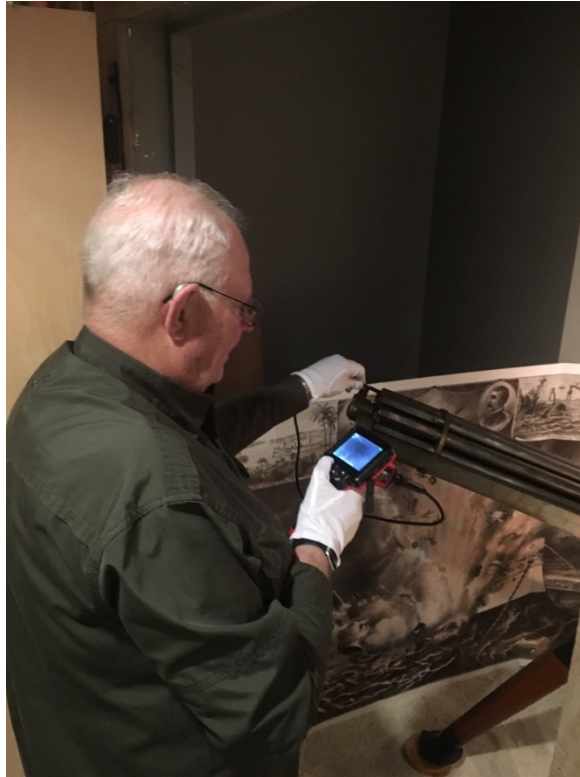
Figure 8. Using the bore light to determine the condition of the rifling on a Gatling gun at the National Firearms Museum.
