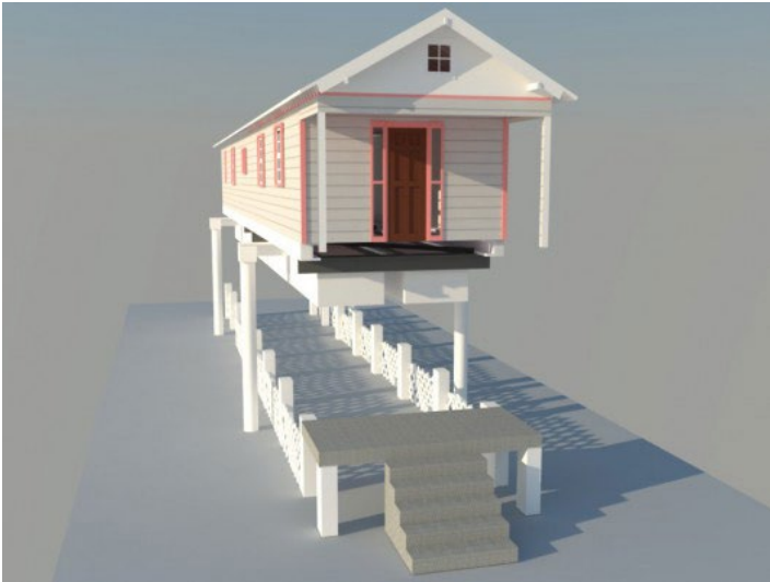
Schematic of what a buoyancy system looks like beneath a shotgun house.
