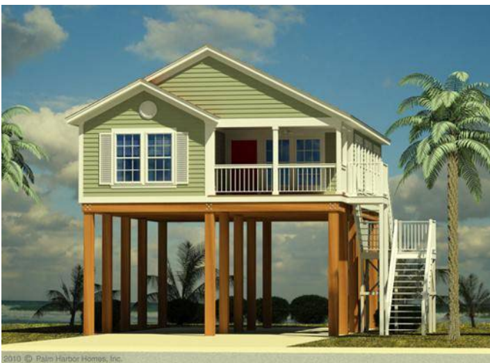
A small wood-frame house elevated on piles.
