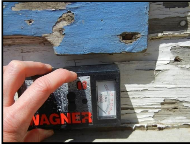
Figure 4.19. Use of a pinless (capacitance) moisture meter to determine the moisture content of siding.
