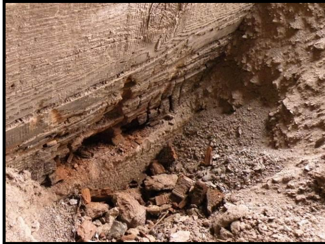
Figure 4.8. Deterioration of wood caused by wood-decay fungi.
