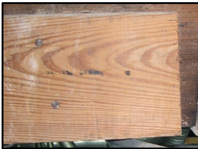
Figure 2.2. Flat-grained board with typical “U” shaped grain pattern.
