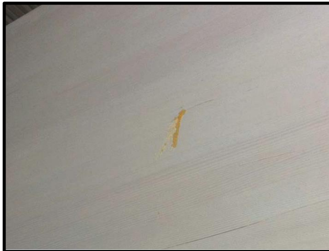
Figure 2.7. Although there is no visible evidence of a pitch pocket on the surface of the wood, the sap indicates the presence of one beneath the surface.
