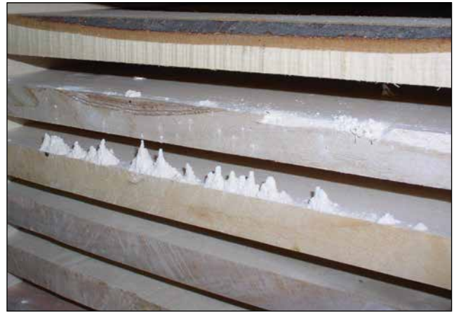
Figure 10—Piles of very fine sawdust are indicative of an active powderpost beetle infestation.
