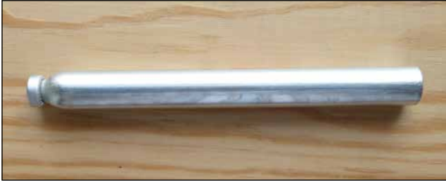
Figure 35—A solid fumigant encapsulated in a metal tube. The cap is removed at installation.
