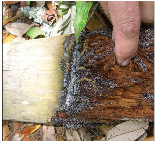
Figure 8—Soft-rot typically occurs under very moist conditions. Photograph courtesy of Anthony & Associates, Inc.
