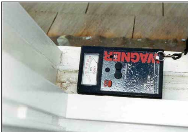
Figure 18—A moisture meter on this window sill shows that the sill is saturated. Photograph courtesy of Anthony & Associates, Inc.
