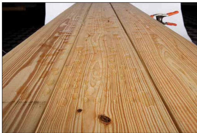
Figure B3—Appearance of EL2-treated wood with incorporated water repellent.
