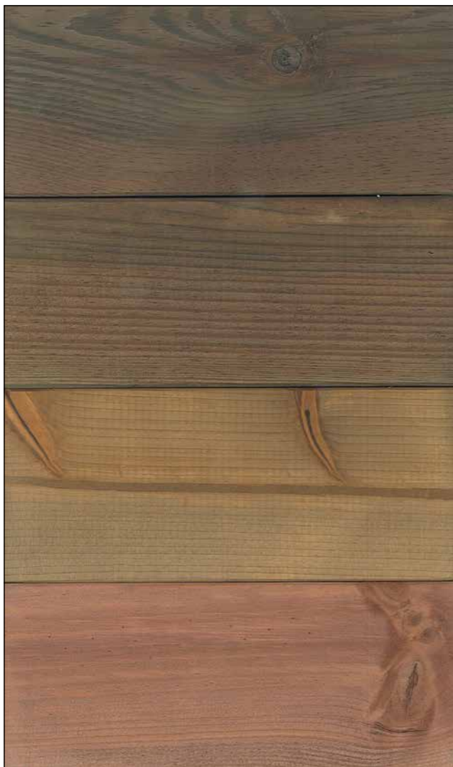
Figure B12—Examples of wood treated with pigmented KDS formulations.
