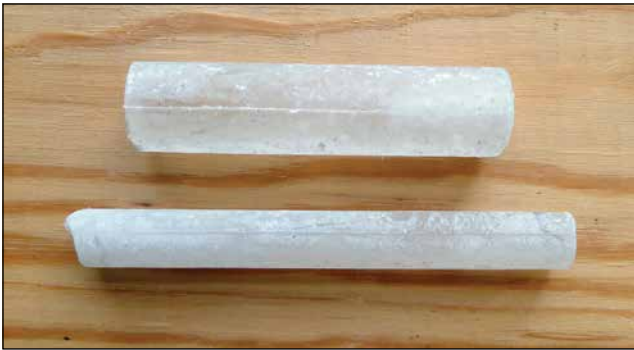
Figure 30—Borate rods are available in a range of sizes including the 19-mm (0.75-in.) and 13-mm (0.5-in.) diameters shown here.
