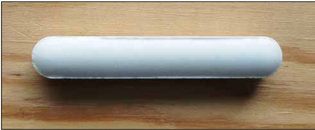
Figure 31—Sodium fluoride rod.
