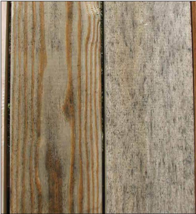
Figure 2—Typical black mold on a softwood (left) and hardwood (right).
