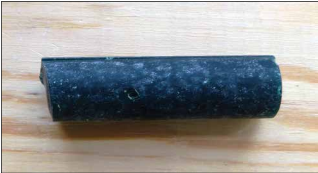
Figure 32—Example of a rod that contains both boron and copper.
