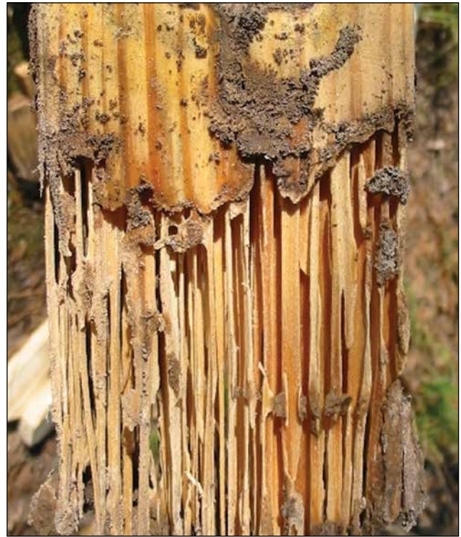
Figure 9—Damage caused by termites after only 6 months of soil contact in Louisiana.
