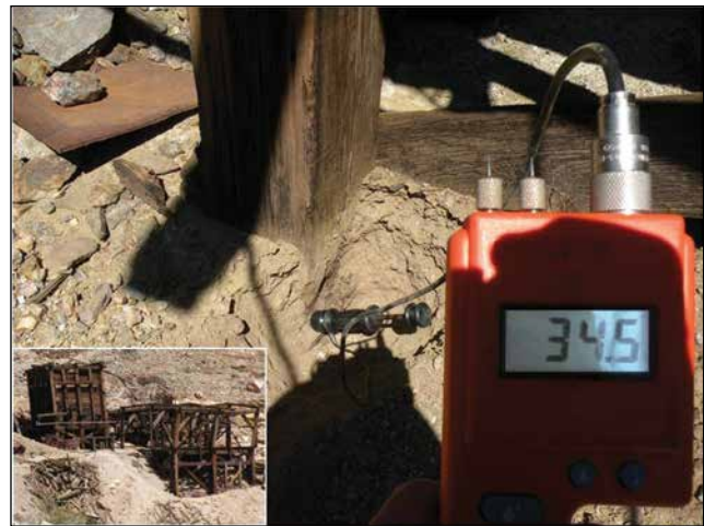
Figure 13—Even in very dry climates, such as Keane Wonder Mine in Death Valley, wood below ground has sufficient moisture for decay. Photographs courtesy of Anthony & Associates, Inc.
