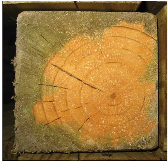
Figure 42—During pressure treatment, preservative typically penetrates only the sapwood. Round members have a uniform treated sapwood zone, but sawn members may have less penetration on one or more faces.
