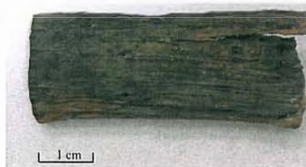
Figure 19. Sample 30d split due to air drying.
