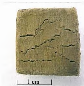
Figure 20. Cracking exhibited by MD sample 89.
