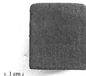
Figure 17 Cross-section of MG sample showing homogenous appearance.
