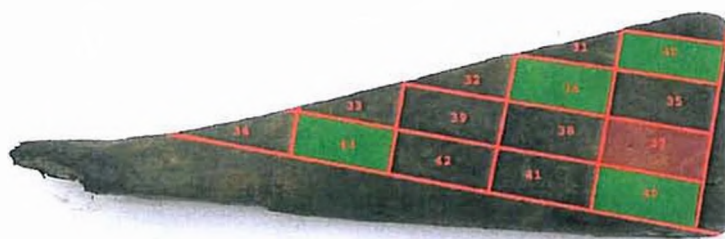
Figure 2. MG-A with overlay of cuts and block assignments. Blocks highlighted in green were used to cut planks. Block 37 (red) was cut into subsamples.
