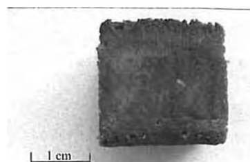
Figure 16. Cross-section of MD block. showing the orange stained exterior and less stained interior.
