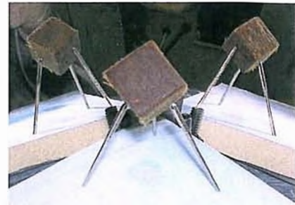
Figure 13. Sample placed on measurement platform in front of mirrors during 3D measurement.
