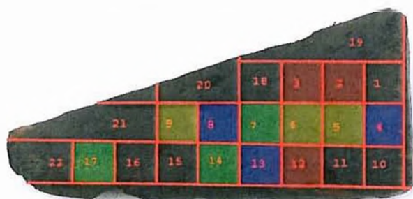
Figure 5. MG-B with overlay of cuts and block assignments. Blue highlighted blocks were cut into subsamples. Green blocks were air-dried. Red blocks were supercritical-dried and yellow were freeze-dried.
