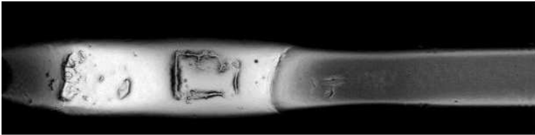
Figure 14. Acoustic image of the hallmarks on a silver Apostle Spoon supposedly dating from 1503.
