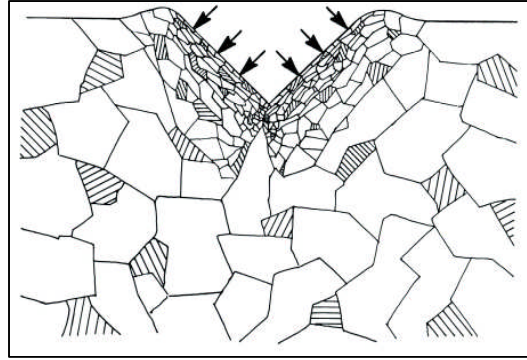
Figure 3. Cross-sectional view of deformation in stamped hallmark. Slip lines, twinning bands, and smaller grain size result where metal absorbs stamping compression (shown by arrows). From Treptow, 1978.
