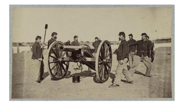
**Figure 14**. A 6.4-inch (16.3-centimeter) caliber, 100-pounder naval Parrott gun mounted aboard the side-wheel gunboat USS *Mendota*. Courtesy of Putnam History Museum. Used with permission.
