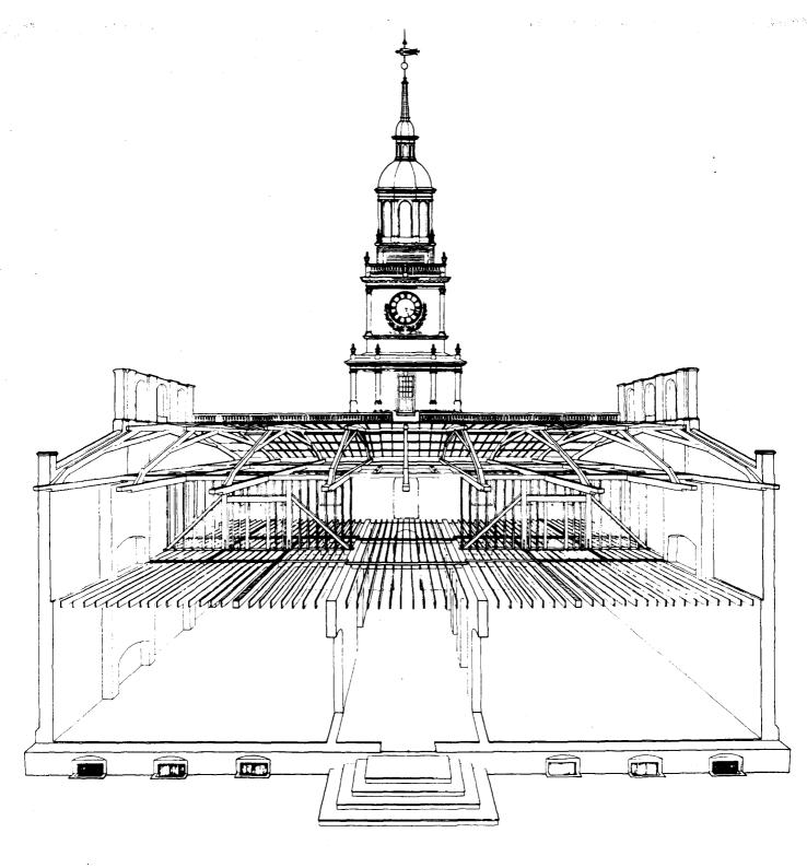
1. Diagrammatic cutaway drawing (from Chestnut Street) showing the principal structural systems.
