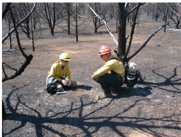
Specialists test for water repellent soil after a wildfire at Zion National Park.
