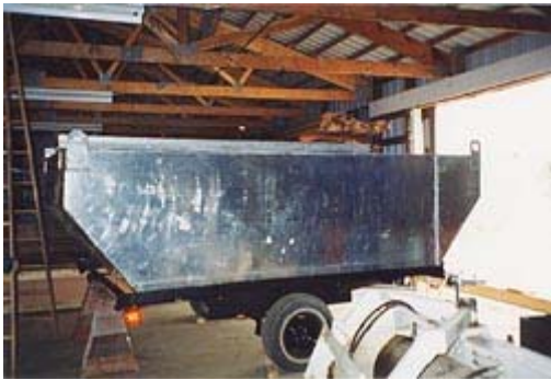
Figure 5. An Army Corps "shop built" barge for use with an airboat to place bales. Lake Sharpe, South Dakota, June, 1994.
