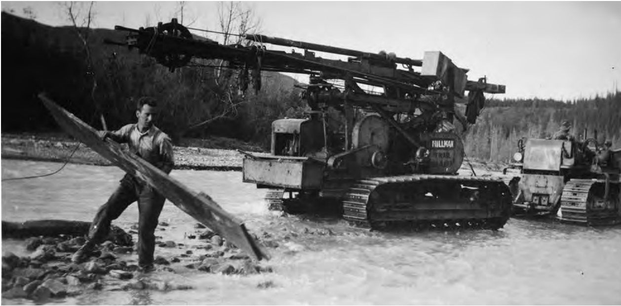
A self-propelled churn drill for finding gold is accompanied across Coal Creek by a Caterpillar tractor crew, ca. 1938. University of Alaska Fairbanks, Stanton Patty Family Papers (2012-93-128).
