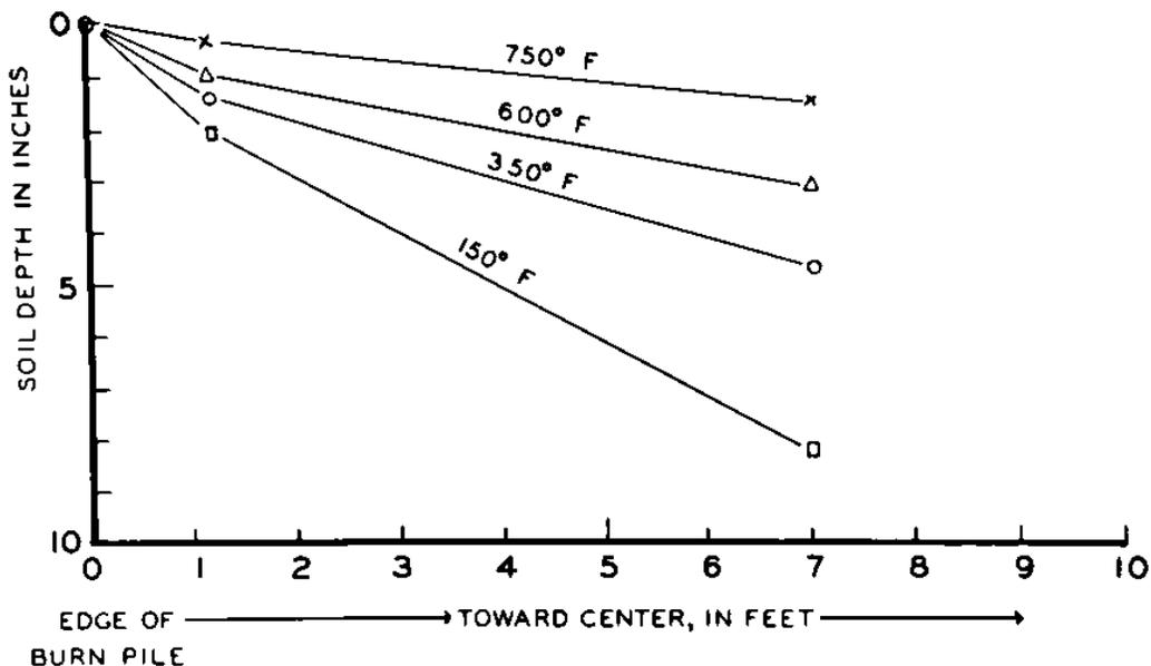
Fig. 4. Heat penetration of soil under burn piles.
