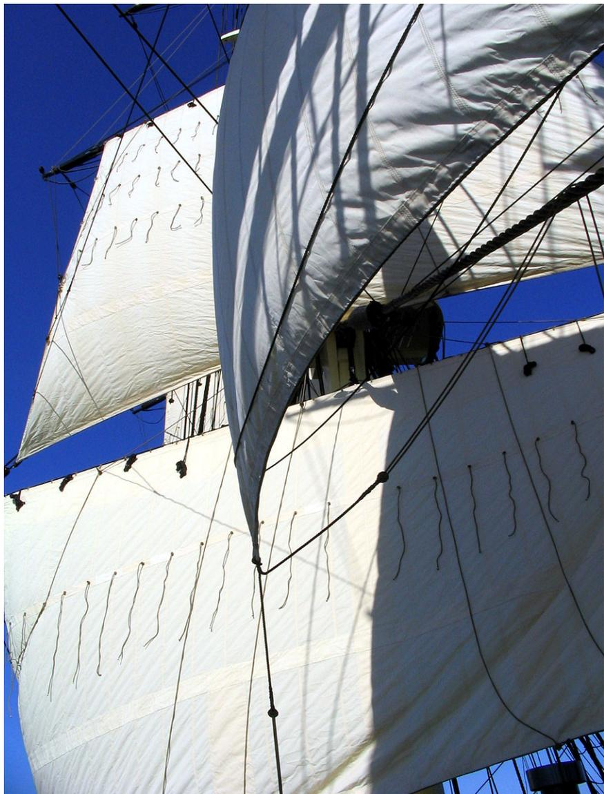
**Above:** the sails of *Friendship*, the replica tall ship at Salem Maritime NHS, are made of modern materials, but replicate the look of the duck that would have been used on the original vessel.
