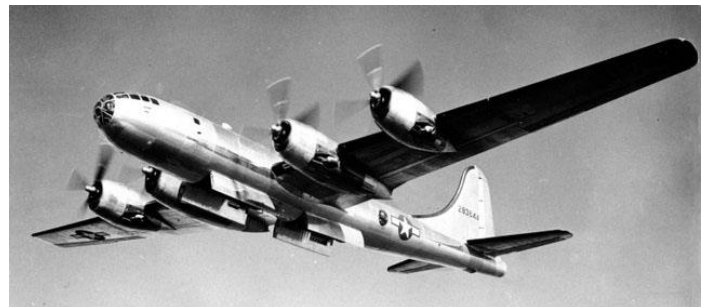
Figure 3. A B-29 in flight with both sets of bomb bay doors open in preparation of dropping its bombs (Photograph courtesy of the Associated Press/Wichita Eagle).
