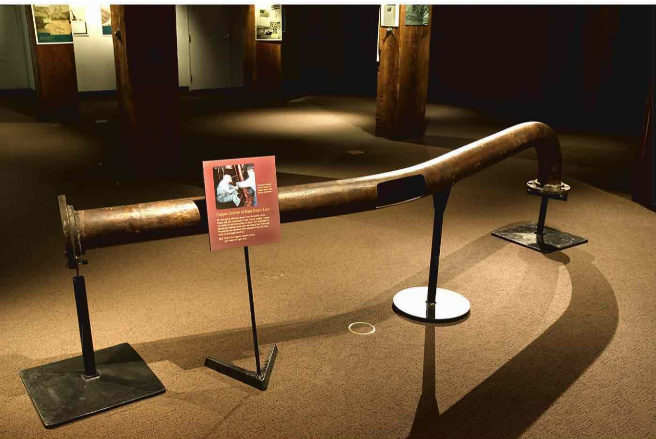
Copper steam pipe removed during restoration. (no collection # at this time)
