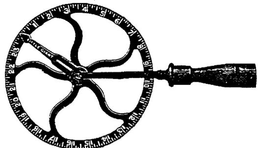
This Wheel has a cherry wood handle; all other parts are made of malleable iron, finely polished. The pointer is held in place by friction, so that it can be set instantly, and will not get loose. The circumference of wheel is exactly two feet, graduated by one-eighth of an inch.
