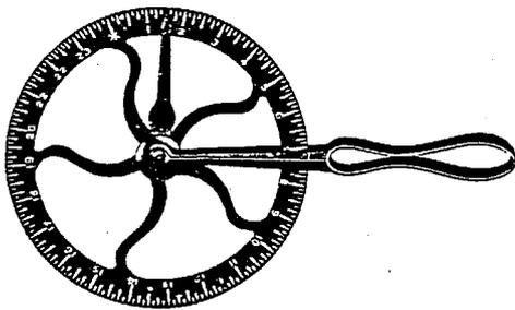
This Graduated Tire Wheel, a drop forging, is made so that the figures and lines are raised above the surface of the wheel and cannot be filled or defaced with rust or dirt; it is a perfect running wheel, turned carefully in a lathe, exactly 24 inches in circumference and accurately graduated.
