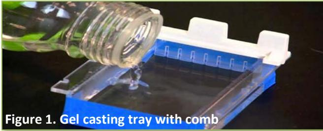
Figure 1. Gel casting tray with comb
