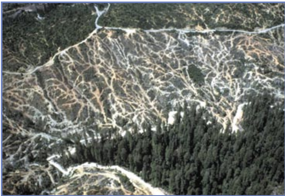
Bond Creek, a tributary of Redwood Creek, in 1978. The web of “skid” roads provided access to individual trees. Once a tree was cut down, a bulldozer dragged (skidded) the log to the nearest landing on a haul road (visible at the top and bottom of this photo).
