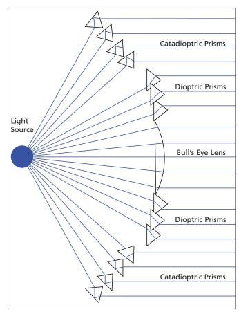
The Fresnel lens works through precise prism and lens alignment, so that the central source light, whether oil lamp or electric bulb, is bent or refracted and transmitted as concentrated parallel beams, making the light visible from farther away. Dioptric prisms bend the light once, while catadioptric prisms bend it twice.
