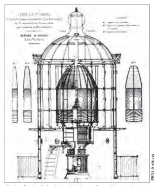
Design for the Point Reyes Lighthouse Fresnel lens and clockworks. This equipment is in the Point Reyes Lighthouse today, although it is no longer in operation.
