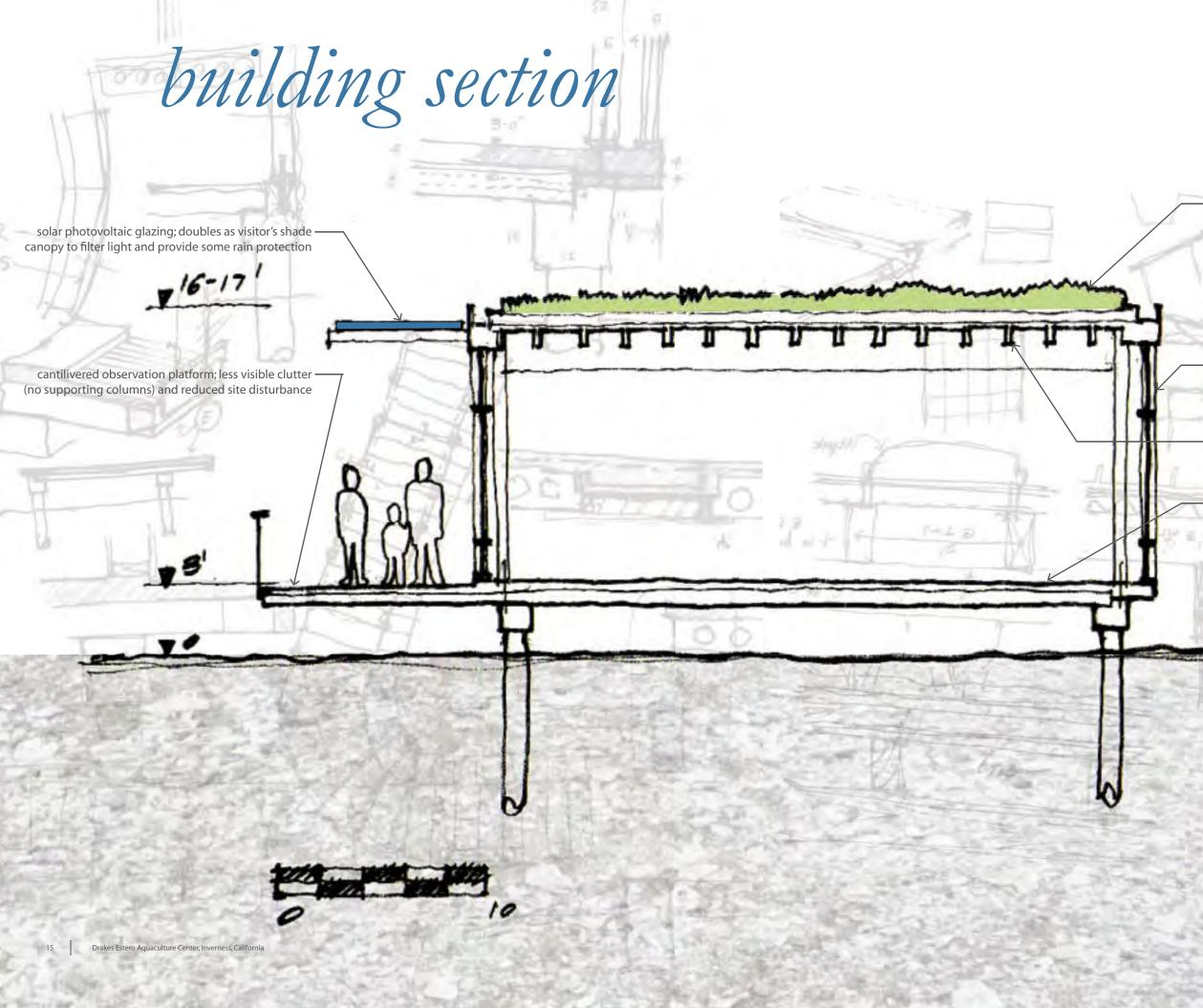
lightweight green roof (solar photovoltaic glazing over the multipurpose work area)
