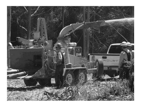
2. Maintenance of Required Roadside Fuel Reduction and Overhead Roadway Clearance. As recommended by the State Fire Code, fuels will be reduced within a ten-foot wide strip along all fire and emergency ingress/egress roads. Not all trees will be removed but trees will be limbed up to 10 feet above ground level. Overhanging
